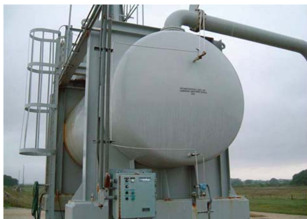
Image 1, 2, & 3: 12" pipe and drums (located adjacent to four brine pits) were treated with CleanWirx, and coated with standard epoxy coating. Equipstar storage facility maintenance project conducted in October 1995 has enjoyed over ten years of maintenance-free durability. This photograph was taken in October 2005. Project demonstrated no corrosion and no coating deterioration. Source: CleanWirx (2006).
